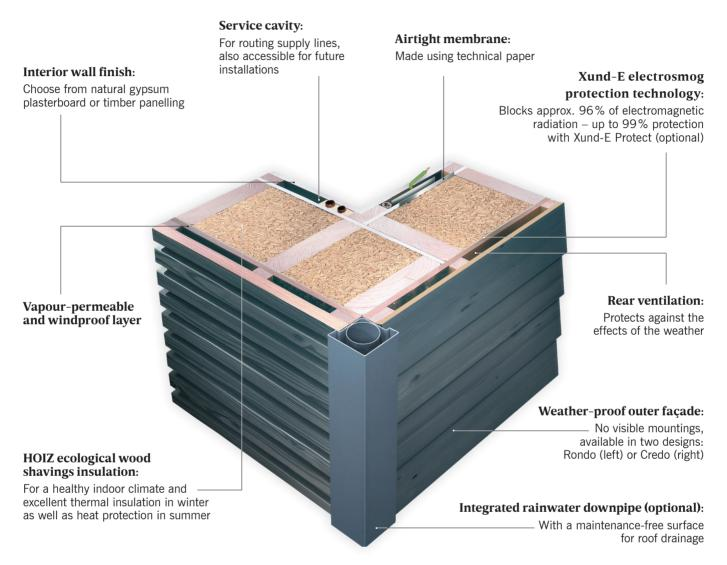
Our Baufritz A wall: 37 cm thick (varies depending on the façade design) energy-efficient wall with U-value= $0.20 \, \text{W/m}^2 \cdot \text{K}$  (or  $0.16 \, \text{W/m}^2 \cdot \text{K}$  with mineral render finish).
