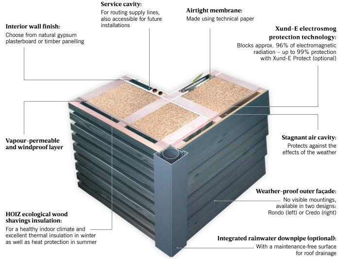
Our Baufritz A wall is 37cm thick (varies depending on the façade design) energy-efficient wall with a U-value of 0.20W/m<sup>2</sup>·K (or 0.16W/m<sup>2</sup>·K with mineral render finish).
