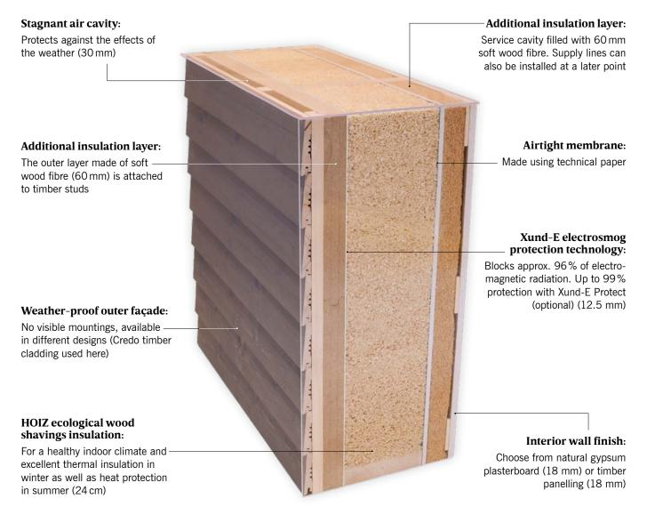
The 46cm-thick Baufritz AAA wall achieves thermal insulation values of a low as 0.13W/m<sup>2</sup>·K Our standard Baufritz A wall is 37cm thick (varies depending on the façade design) and is for use in PlusEnergy, solar or passive houses with a U-value of 0.20 W/m<sup>2</sup>·K (or 0.16 W/m<sup>2</sup>·K with mineral render finish). Subject to modifications.
