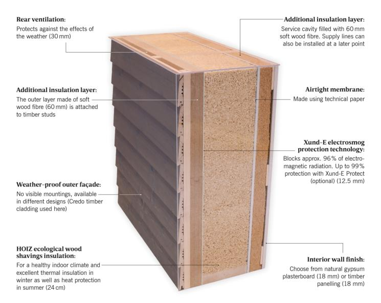
The 46 cm-thick Baufritz AAA wall achieves thermal insulation values of a low as 0.14W/m²·K Our standard Baufritz A wall is 37 cm thick (varies depending on the façade design) and is energy-efficient with a U-value of 0.20 W/m²·K (or 0.16 W/m²·K with mineral render finish). Subject to modifications.
